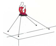
Lifting with 4 points: use 2 load positioners
